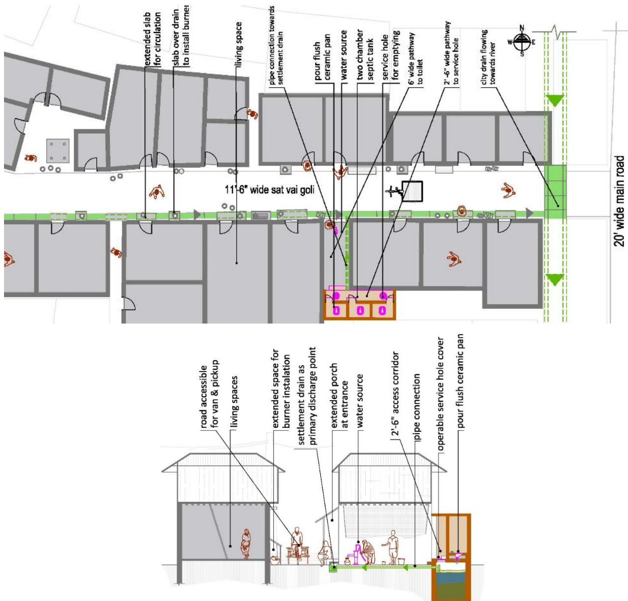
Figure 4.12: periodic FS discharge from shared toilet with septic tank (20 HH; 1 alley) (R-6), sat vai goli
